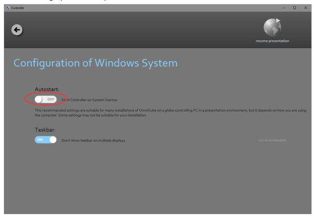
Disable "Start Controller on System Startup" in the "Windows System" category to remove the previous autostart. Then enable the property again to activate the automatic start of OmniSuite's Controller.
